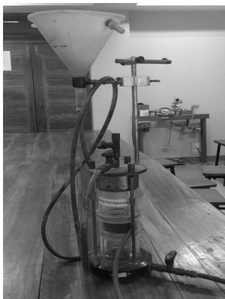
**Figure 8.1 Permeability Apparatus**
