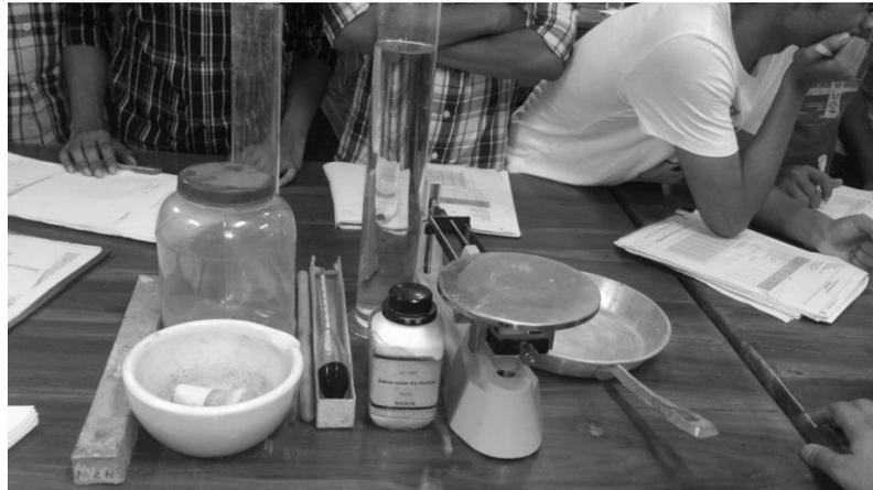
**Figure 4.1 Hydrometer Test Apparatus**
