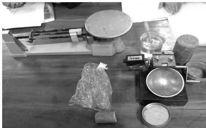
**Figure 7.3: Atterberg Limit Test Apparatus**
