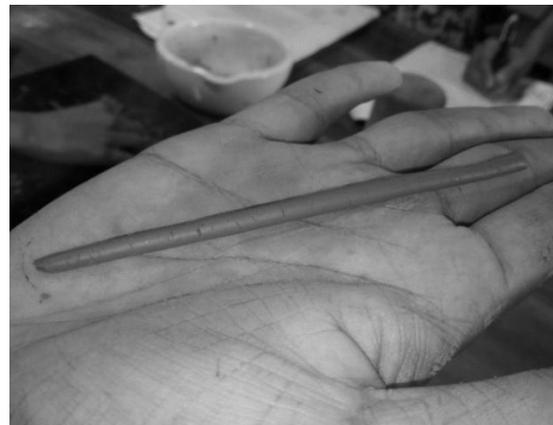
**Figure 1.4: Toughness and plasticity Test**
