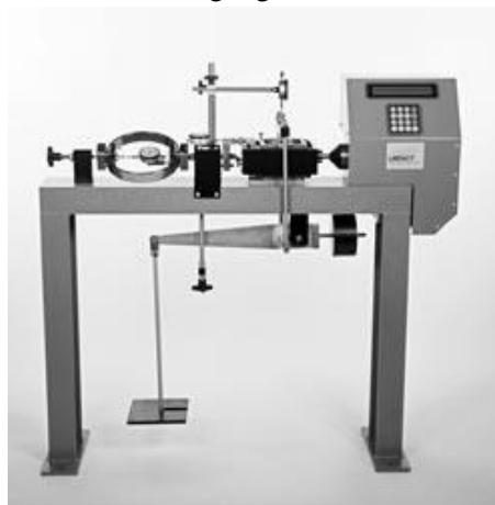
**Figure 11.1 Direct Shear Test device of the laboratory**
