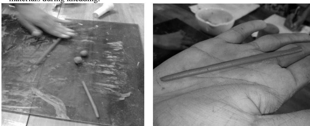
**Figure 1.4: Toughness and plasticity Test**
