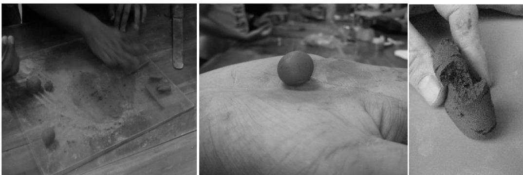
**Figure 1.3: Dry Strength Test****Table-1.3 Dry Strength**
