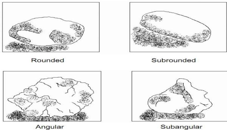
**Figure 1.1 Shapes of coarse-grained soil particles**
