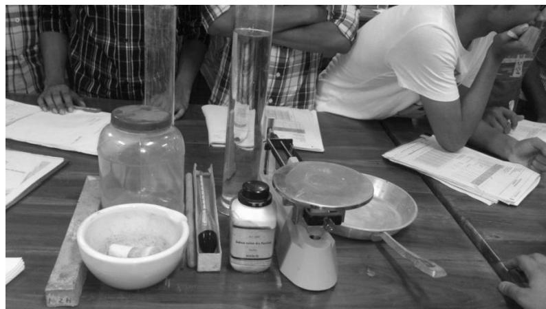
**Figure 4.1 Hydrometer Test Apparatus**
