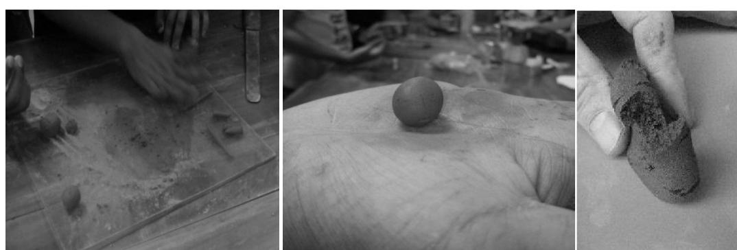
**Figure 1.3: Dry Strength Test****Table-1.3 Dry Strength**
