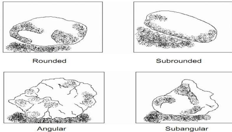
Figure 1.1 Shapes of coarse-grained soil particles
