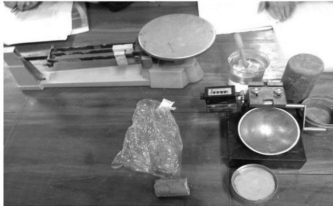
Figure 7.3: Atterberg Limit Test Apparatus
