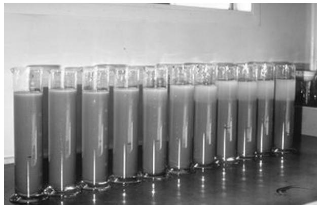
**Figure 1.2: Dispersion Test****2. Dry strength:**
