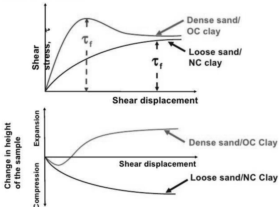
Figure 11.2 Stress-strain relationships of sand (Direct Shear Test)
